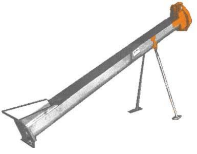
The auger turns in a flange bearing at the drive end and uses an ultra-high density polyester bearing at the lower end, with no hanger bearing in between to obstruct flow. Since the lower bearing is UHMW plastic, we do not recommend sand to be used as bedding material because of its abrasiveness. The drive unit features a heavy-duty Belt-Chain jackshaft drive with #50 Roller chain. A 5-10 hp motor is all that is required to handle your heaviest manure loading needs.
